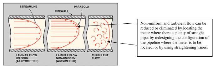
Figure 3. Laminar and turbulent flow.
