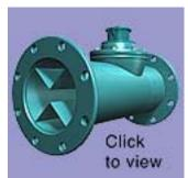
**Figure 7.** Example of a typical flanged meter with straightening vanes.
