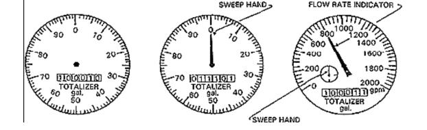
Figure 2. What a mechanical meter head might look like and what readings are provided. For agricultural applications, totalizing in acre-feet is best.
