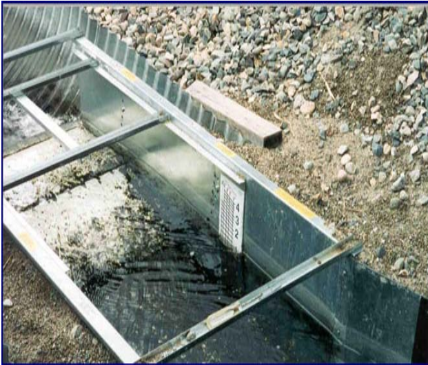
Figure 14. Long-throated ramp flume with direct read on staff gauge in cubic feet per second.
