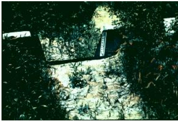
Figure 10. Weir pool is full of sediments, preventing the water from pooling correctly behind the weir for accurate measurement
