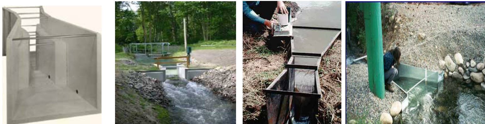
Figure 18. Parshall flume before installation and in-place and measuring water.
