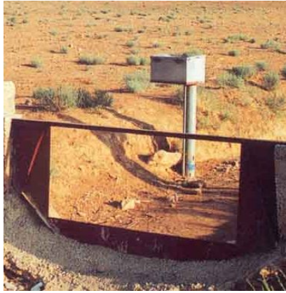
Figure 5. Example of fully-contracted rectangular weirs (note that h_o is the head (or depth) of the water flowing over the weir). This type of rectangular weir requires a weir blade with sides.
