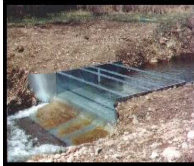
Figure 14. Long-throated ramp flume with direct read on staff gauge in cubic feet per second.
