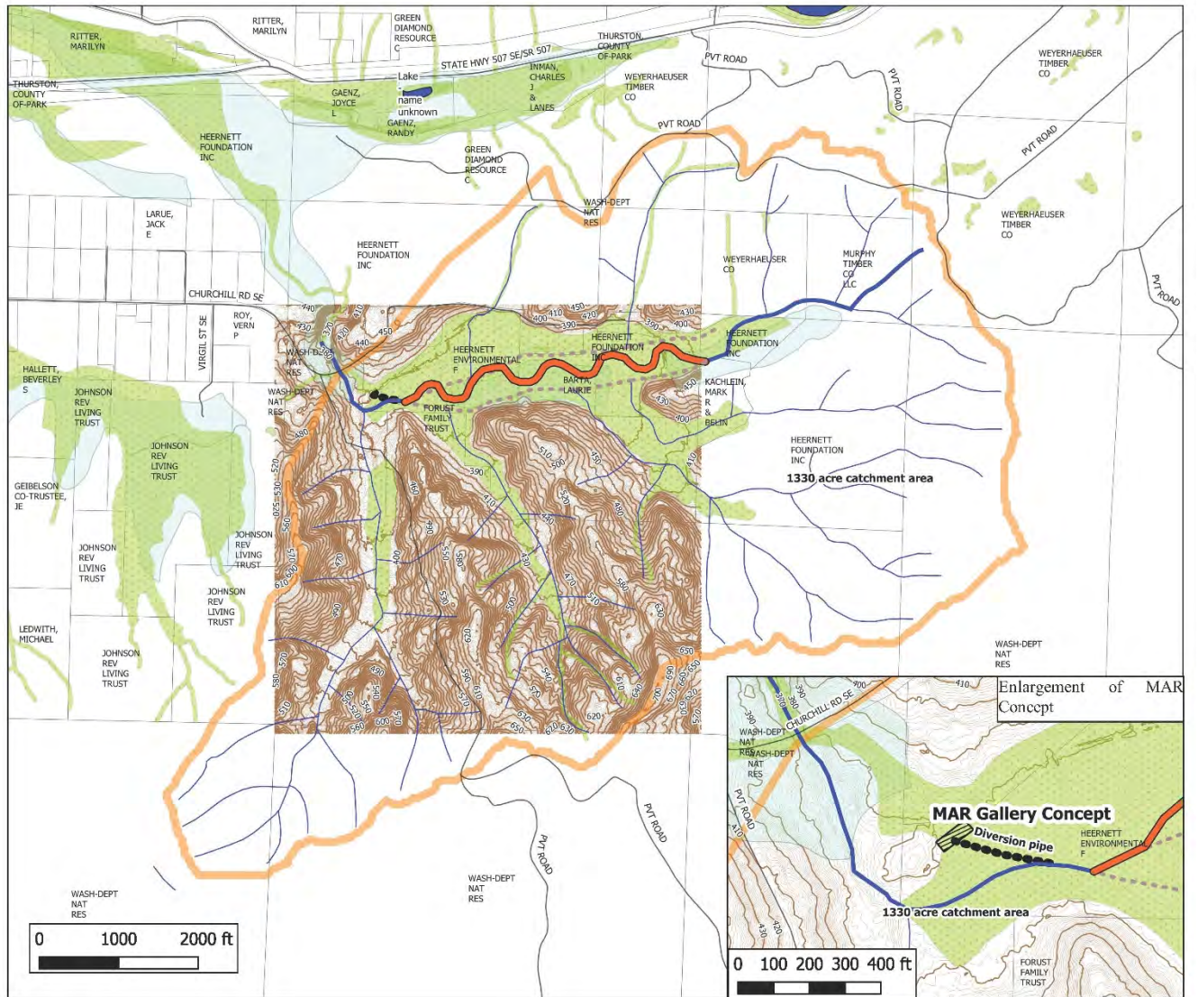
Figure 2 – Project Area showing conceptual ditch removal and stream re-meandering with a possible Managed Aquifer Recharge (MAR) site fed by ~1330 acres of catchment:
