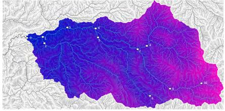
VELMA model domain for the Mashel Sub-basin showing the stream network, simulated gages at key reaches and boundary view (McKane et al, 2018).
