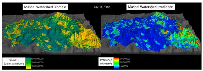
**Figure 15.** Penumbra model simulation of solar irradiance reaching ground and stream surfaces across the 84 mi<sup>2</sup> Mashel River watershed, after accounting for topographic and object (forest) shading.
